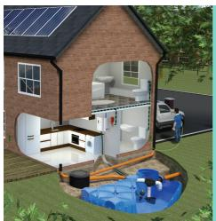
With the average home owner using around 150 litres of water per day, the StormSaver rainwater harvesting system will enable the metered home owner to recycle rainwater and potentially reduce their bills by up to 50%, whilst remaining kinder to the environment. StormSaver can also alleviate pressure on local drainage in line with Sustainable Drainage Schemes (SuDS), to help prevent flood risk.
