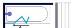
A: Moving Panels (screen width when folded into the bath 226mm) B: Fixed Panel
