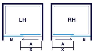
Sliding Door in Recess
