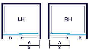
Sliding Door in Recess
