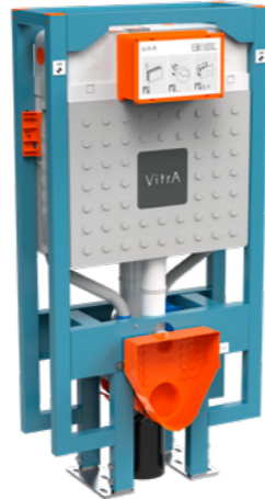
Regular wall-hung frame, 8cm, back-to-back fixation with electrical connection, 3/6 litre £700 - 768-5850-01 H: 1120mm W: 555mm P: 200mm
